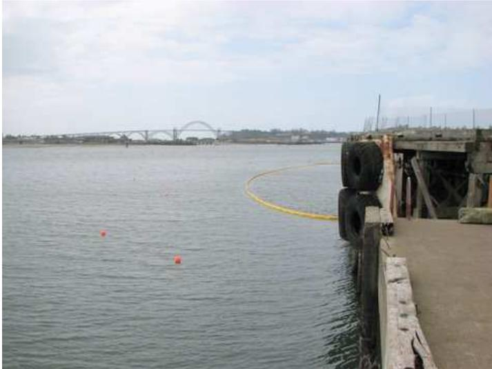
Oil Boom Deployed at the Terminal
