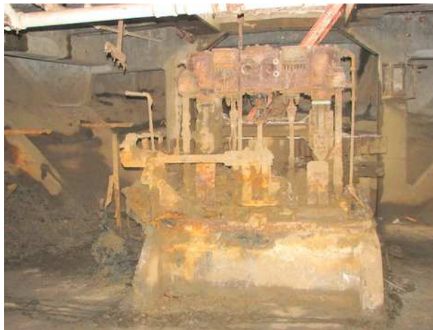
Below decks on the Pasley 1943 steering gear and twin cylinder, vertical reciprocating steam engine
