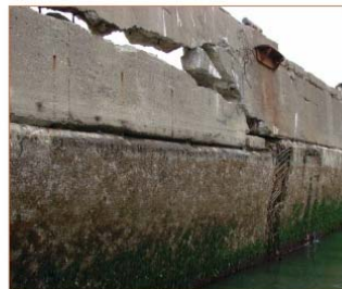
Note the cracks and the spalling in the hull of the Pasley.
