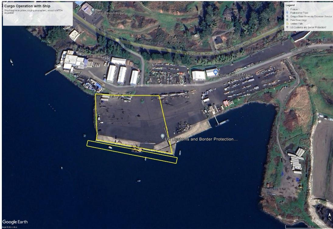
This is a hypothetical scenario for a cargo ship operation at the Terminal. The ship represented here is a Handy size vessel, approximately 600' in length, with a 75' beam. The ship would likely "hang over" the end of the pier, in which case we will encounter challenges with hoist access at times the ship is in port. Some of the ways we could face this challenge are suggested above; while the ship is in port, we would likely be limited to smaller vessels using the hoist.
